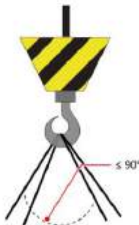
Figure 2-6 Schematic Diagram of Cable Angle for Lifting Operations
