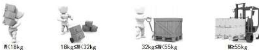
Figure 2-3: Schematic of Lifting Methods for Different Weight Loads
